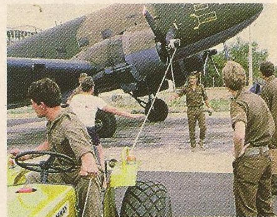
ABOVE: When a Dakota's engine won't start on its own power, you wind it up and pull it into activity with a tractor. This procedure, photographed at Ondangwa Airport, was a daily occurrence with one of the recalcitrant old girls.
